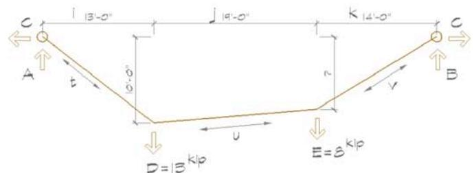
Using Pythagorean theorem we can solve for tension of cable "t"
