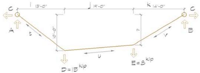
Knowing that each node should have a sum of forces equal to zero, we can solve for the tension "u" in the cable by solving for either node "D" or node "E". Let's take node "D" and solve the angles, and then based on  $F_x=0$  solve for tension "u" in the cable:
