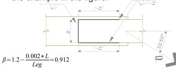
$$\varphi R_n = \varphi * F_{nw} * A_{we} = 0.75 \left[ 0.60 * F_{EXX} * (1 + 0.5 * \sin^{1.5} \theta) \right] * \left[ \frac{\sqrt{2}}{2} \beta * L * Leg \right]$$
